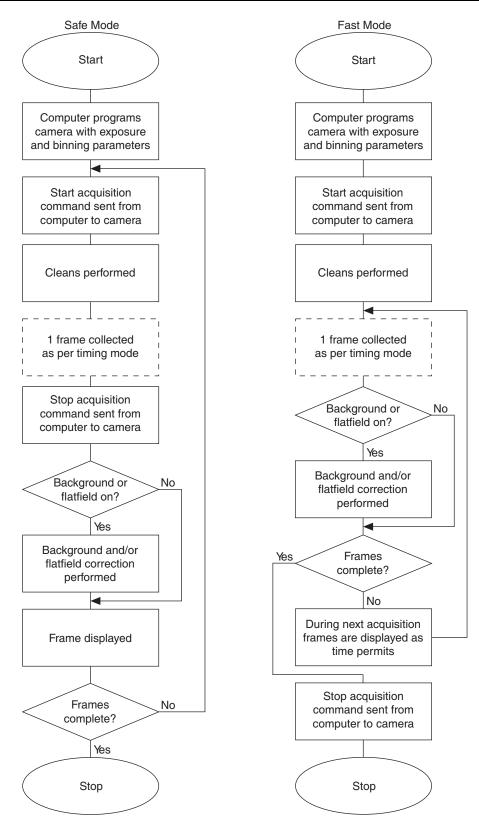
Figure 9. Flowcharts of Safe and Fast Mode Operations
